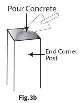
2. Now fill the posts with concrete, tapping on the sides of the post to remove air-pockets in the concrete (**Fig.3b**).
