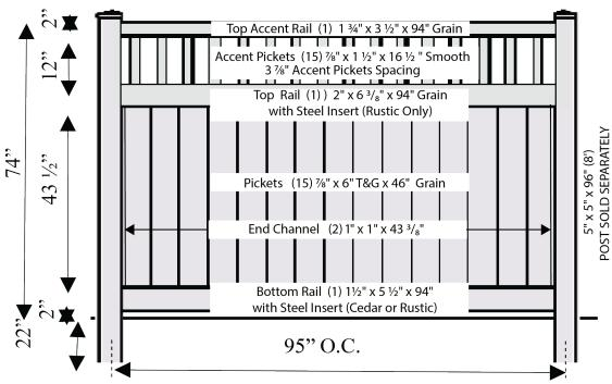
Cedar with Bottom Rail Steel Insert Only Rustic with Top and Bottom Rail Steel Insert
