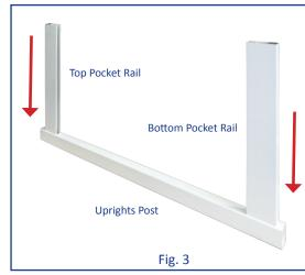
Insert both the Top & Bottom Pocket Rail all the way into the Uprights Post. (Fig. 2 & 3)
